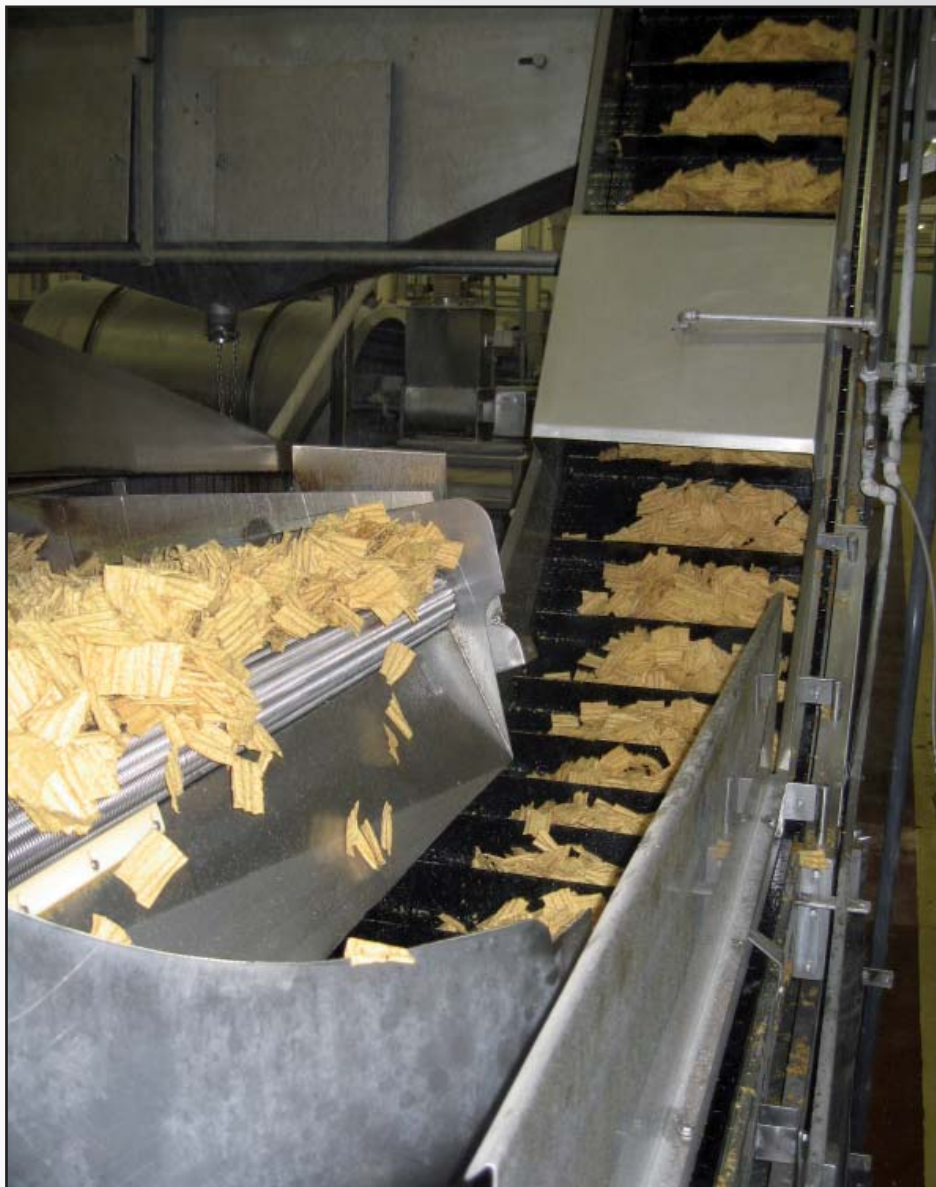
INCLINED CONVEYOR FOR CHIPS FTR2015 BELT
