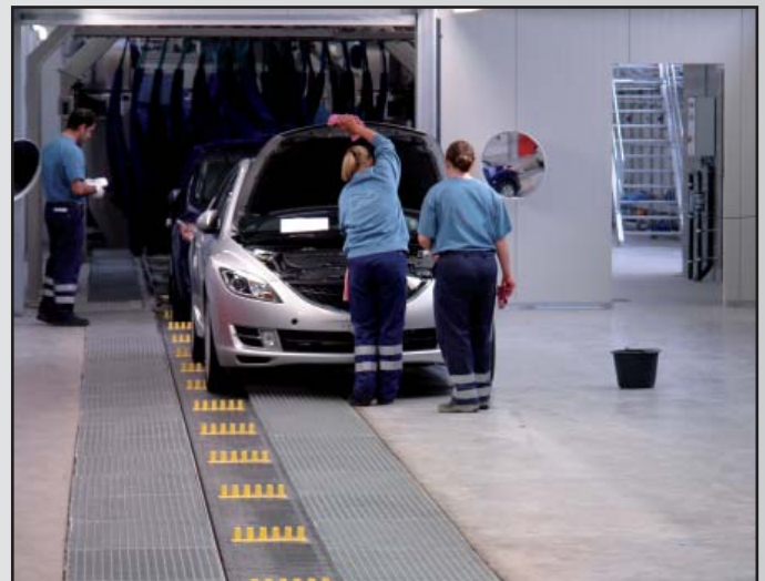
3125 END OF LINE INSPECTION BELT CONVEYOR WITH T2 DIN PUSHERS
