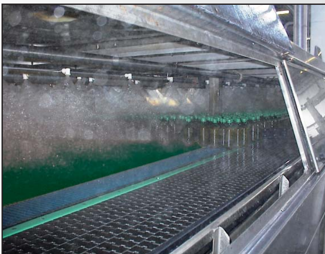
GLASS BOTTLE WARMER WITH 2000 RAISED RIB BELT AND DTS-C TRANSFER
