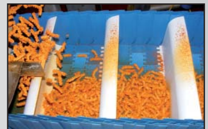
INFED OF INCLINED CONVEYOR WITH 2010 ISR6
